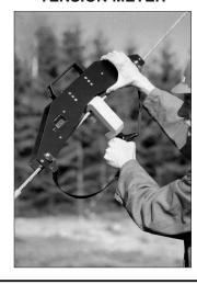
RTM Specifications: 2 ton to 20 ton Capacity 1/4" to 1 1/2" Wire Rope
