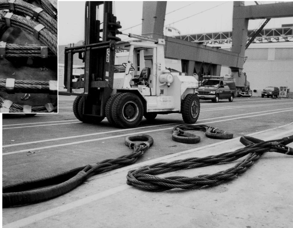
Follow OSHA, ANSI B30.9 and Manufacturers Guidelines. Can fail if damaged, misused or overloaded. Inspect before use. Use only if trained. Do not exceed rated capacity. Protect sling from contact with edges. DEATH or INJURY can occur from improper use or maintenance.
