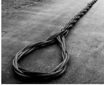
with riggers in the field that wished to create a sling for heavy lifts that could be visually inspected and have the highest flexibility possible in a Multi-Part wire rope sling.
