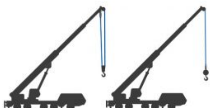
Hoist & Aux Rope
